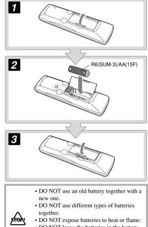
• DO NOT leave the batteries in the battery compartment when you are not going to use the remote control for an extended period of time. Otherwise, the remote control will be damaged from battery leakage.
